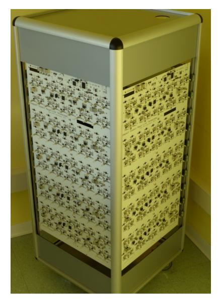
Two monolithic boards serve as readout, trigger logic and to monitor the working parameters
