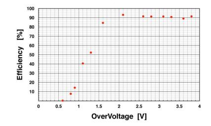
The efficiency of a channel reaches 90% when an overvoltage of  $\ge 2V$  is applied.
