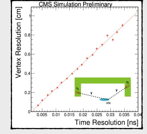
~30ps TOF resolution on high energy photons allows to identify diphoton production vertex with precision better then 1cm Informations extracted from each MCP waveform
