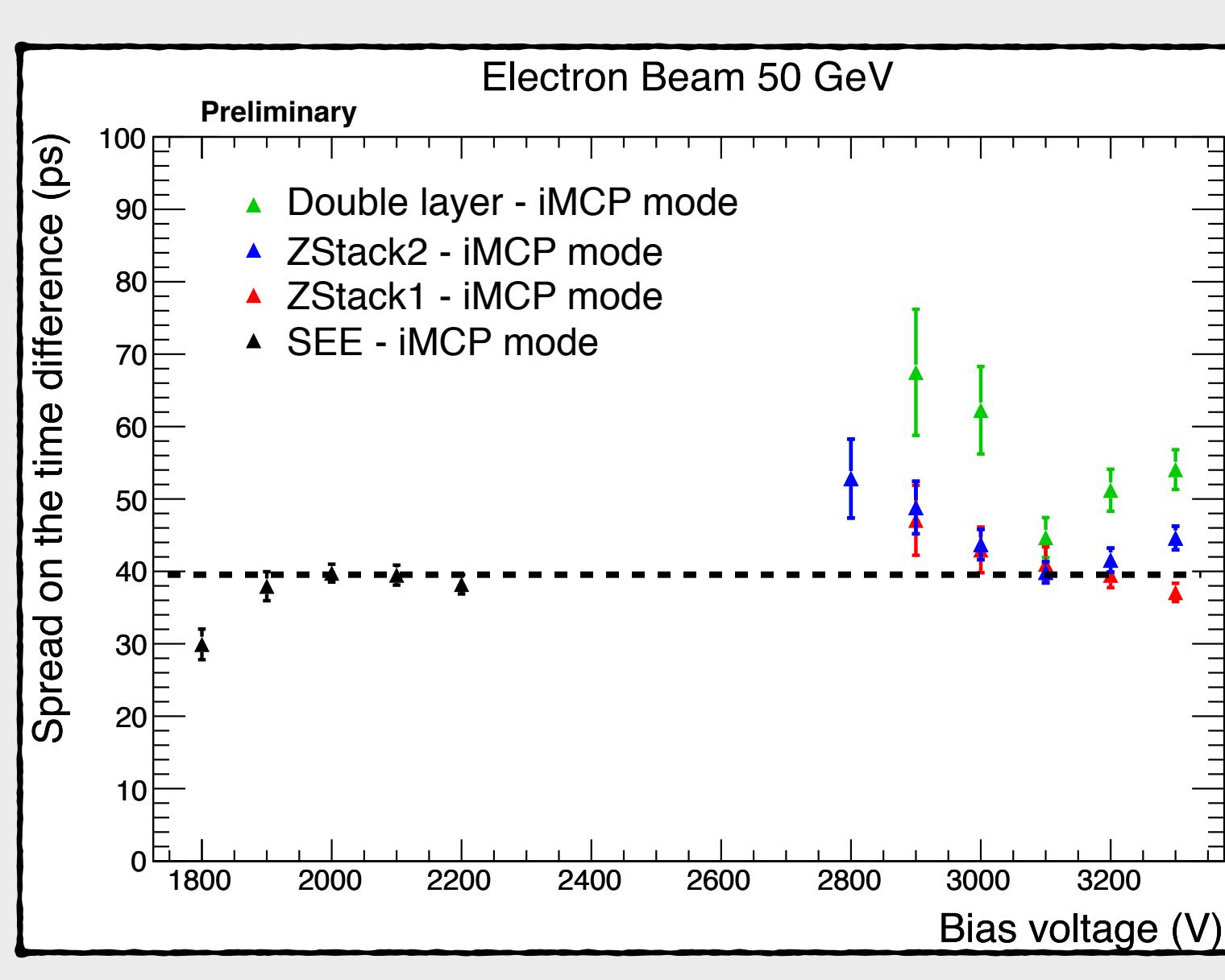
**σ(t<sub>TRIG</sub>-t<sub>MCP</sub>) ~ 40 ps for Z-stack & enhanced SEE:**
