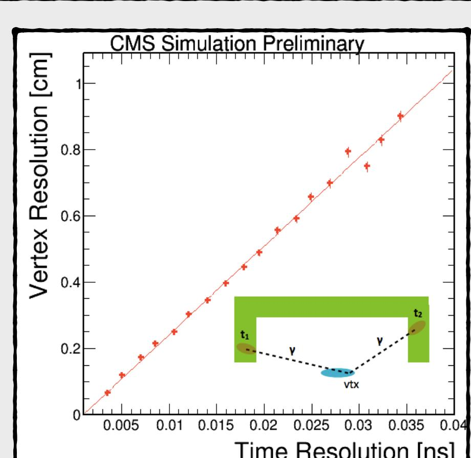
~30ps TOF resolution on high energy photons allows to identify diphoton production vertex with precision better than 1cm
