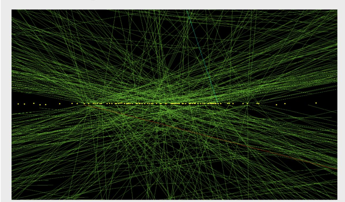
Pile-up at hadron colliders: several interactions per bunch-crossing. LHC Run1 ~ 25 PU
