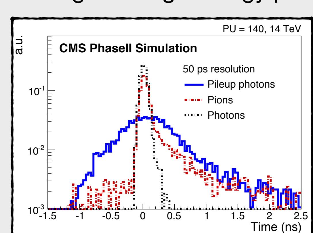
Already 50ps TOF resolution sufficient to get a good rejection in forward EM calorimeter for pile-up photons
