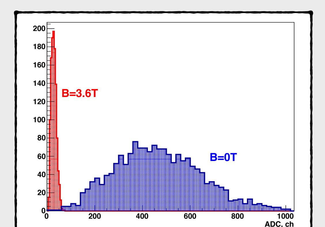
**Moderate loss up to 3T, bigger losses beyond that: loss ~ factor 15 for axial field @ 4T**
