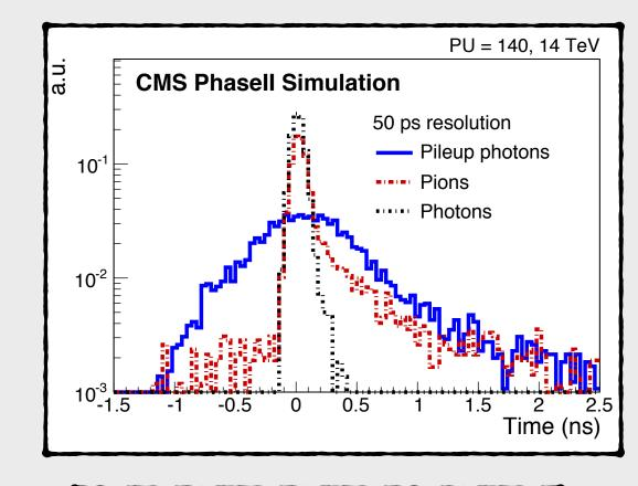
Already 50ps TOF resolution sufficient to get a good rejection in forward EM calorimeter for pile-up photons
