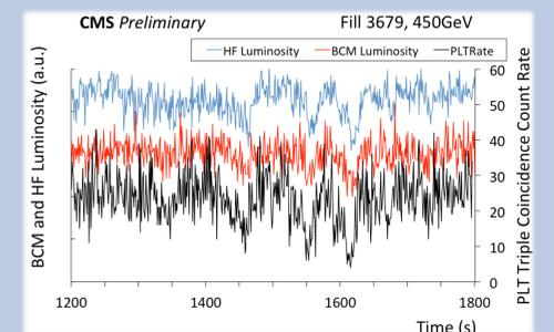
Qualitative comparison of luminosity measurements done by HF lumi, BCM and the PLT during a luminosity scan of the LHC
