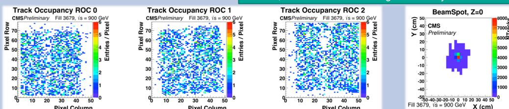
Track occupancy plots from a single PLT telescope from reconstructed tracks measured during non-stable collisions in CMS
