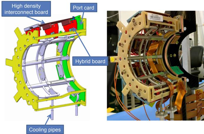
A design drawing of a PLT carriage equipped with a single telescope and a picture from the final detector quarter with all four telescopes and electrical connections in comparison
