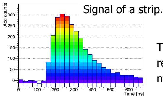
The TGD prototype was exposed to cosmic rays. The detector was read-out with 2 APV-25 chips and operated with an Ar:CO<sub>2</sub> 93:7 gas mixture.
