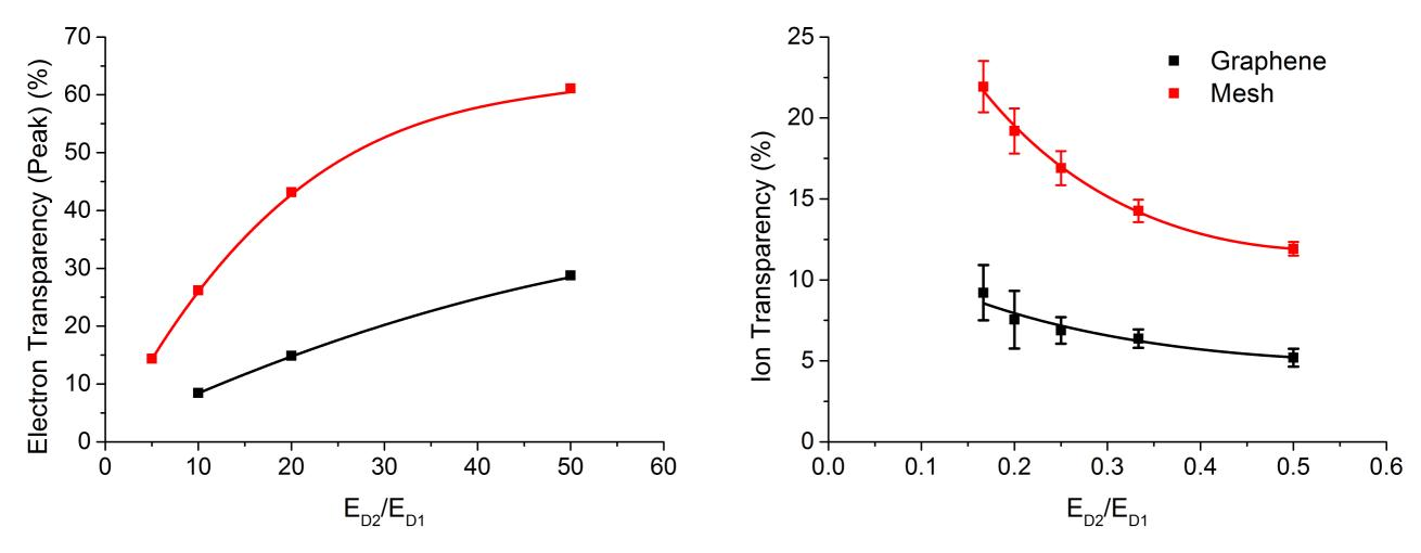
Reduced the electron and ion transparencies Same behaviour of very small optical transparency mesh Measurement is dominated by defects on graphene
