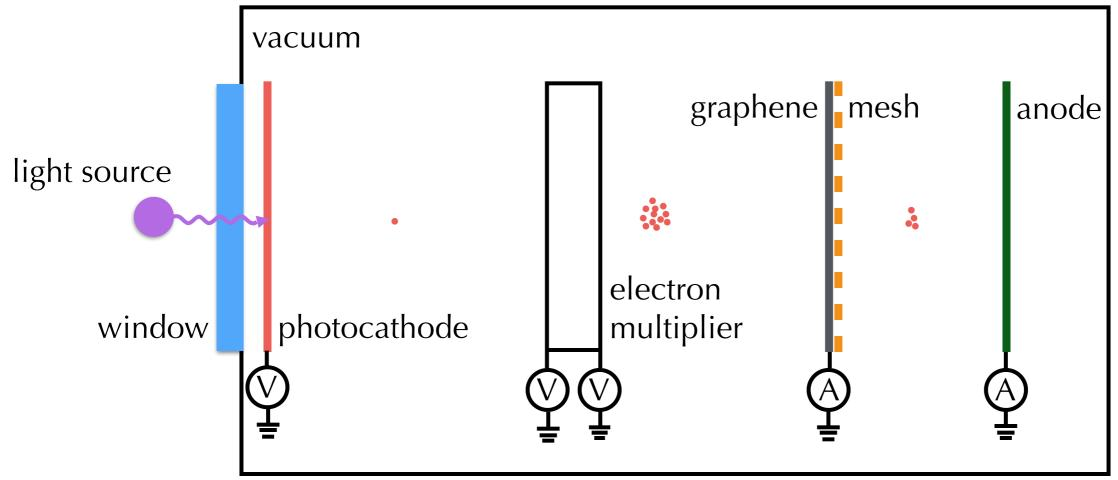
Electron multiplier may be not needed if the light source is strong enough **Tune** the electron **energy** at the eV scale XIII Pisa Meeting on Advanced Detectors - Isola d'Elba - 24-30 May 2015
