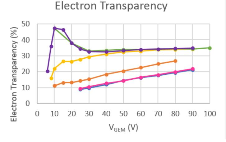
Graphene on top of a GEM Ar/CO<sub>2</sub> 70/30 E<sub>D1</sub> = 50V/cm, E<sub>D2</sub> = 1kV/cm X-ray beam (collimated and not) **Tri-layer not transparent to electrons** Graphene *shorted* the GEM electrodes
