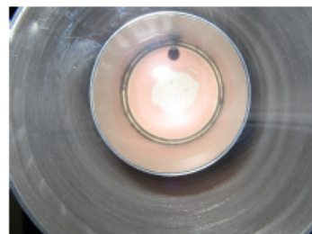
Empty cell before liquefaction. The hydrogen gas inlet is visible
