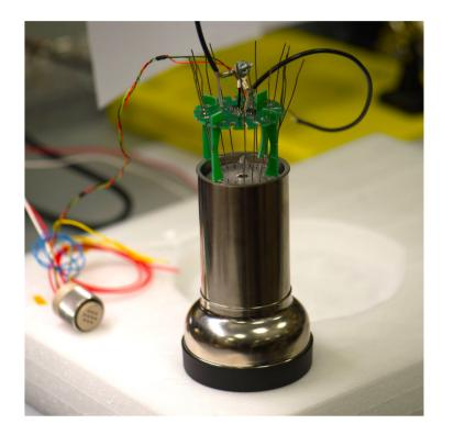
cryogenic environment (i.e. Liquid Argon, LAr, or Liquid Xenon, LXe). The board requires a current supply for the amplifier stage and an high voltage input to power the PMT. 1X and 10X amplified signal outputs are provided.
