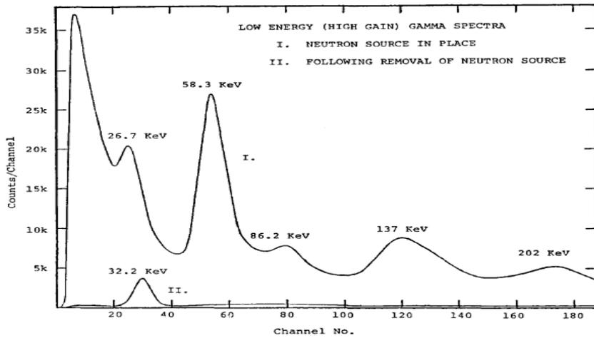
Typical gamma spectra obtained with NaI. Spectrum I, was collected when  $^{256}\text{Cf}$  neutron source was in place, Spectrum II, was obtained after the removal of the neutron source.
