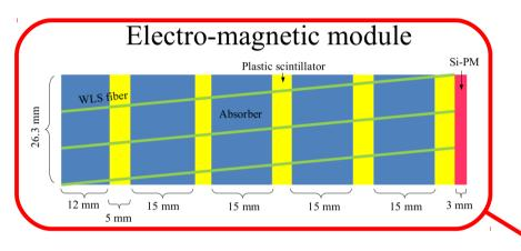
Radial views (the  $2\pi$  geometry is obtained with 76 azimuthal modules)
