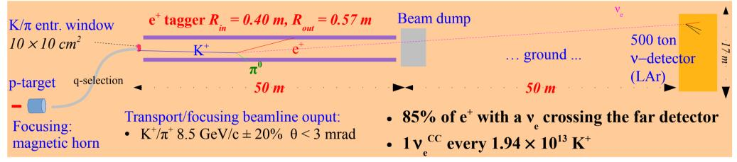
v flux proportional to the e<sup>+</sup> rate in the tagger v flux will NOT depend on hadro-production, K/ $\pi$ production ratio, Protons on Target (PoT), 2<sup>ry</sup> beamline efficiency but only on: the geometrical acceptance of the e<sup>+</sup>-tagger/v-detector, the e<sup>+</sup> tagger efficiency and the mastering of residual backgrounds. O(1%) systematic error achievable
