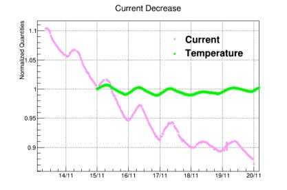
Since the gas system keeps the absolute pressure of the chamber fixed, the gas status was monitored by measuring temperature through a Pt100 sensor. **Current oscillations induced by temperature variations** were removed offline. Since gas gain has a power dependence on temperature and pressure with opposite power indices
