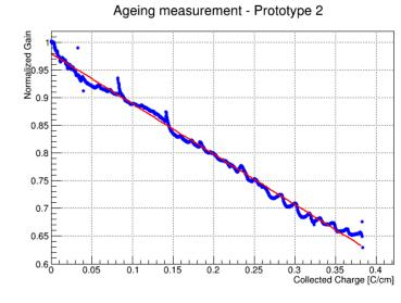
In the central region of the hottest wire the gain loss is about **16 %/year**, while in most wires the gain loss is below 10%/year. This can be easily recovered with a small increase in the high voltage of the wires.
