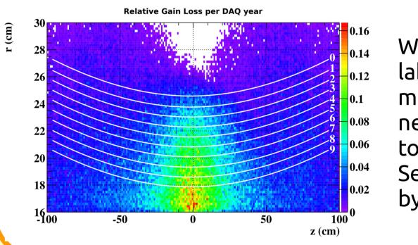
We performed laboratory tests to measure the **robust**ness of the chamber to **ageing effects**. See the poster by M. Venturini.
