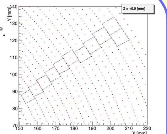
The detector geometry will be realised by the stacking of FR4 wire PCBs with PEEK spacers in each sector of the endplate. A carbon fiber support structure will guarantee the proper wire tension. In the inner side an aluminated mylar foil will tight the gas volume. All the mechanical compatibilities and the insertion in the MEG II apparatus will be checked with a mock-up chamber.
