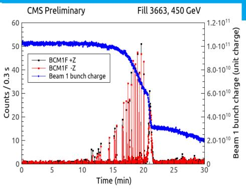
This is an illustrative plot. The BCM1F detector counting rates during a beam loss. The beam intensity as a function of time is shown in blue. The count rates of the BCM1F detectors are shown in red and black. At the time when the beam loss starts the count rates of BCM1F detectors are rapidly growing:
