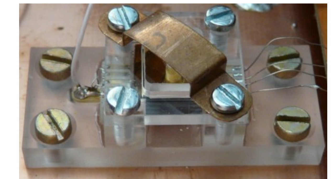
Fig.5: Assembled detector stack as used in the test beam at DESY-II.
