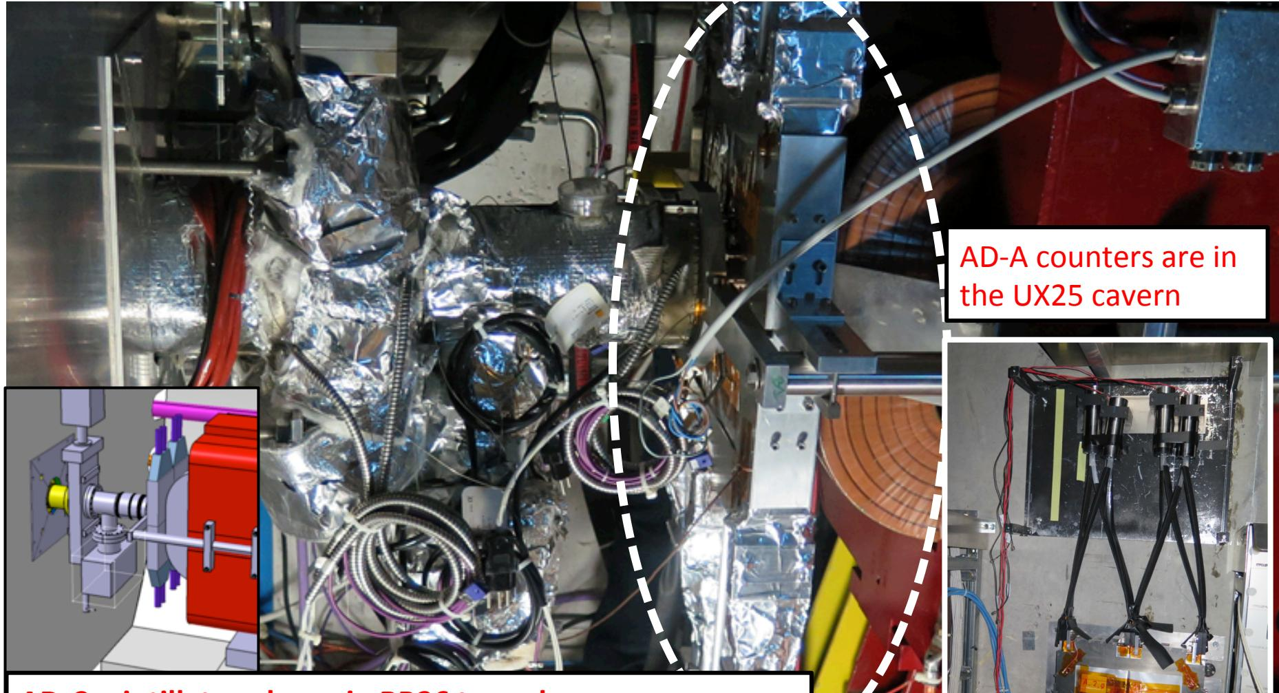
**AD-C scintillator planes in RB26 tunnel**
