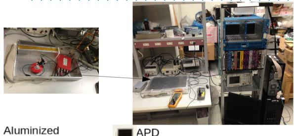
A scintillation counter consisting of a pure CsI crystal (6x6x30 cm<sup>3</sup>) photodiodes avalanche and S8664-1010 (Hamamatsu and. S8664-55) is studied.
