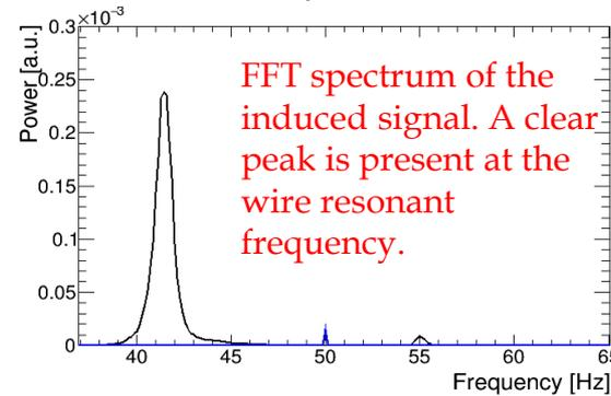
A **sinusoidal HV based** system developed by INFN Lecce
