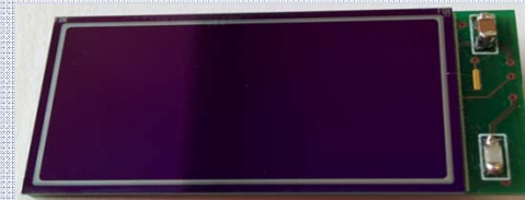
Picture of the detector mounted in a proper carrier (back side view)
