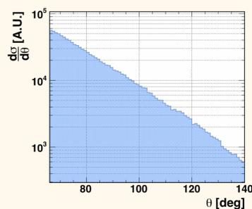
Figure 4: Simulated Mott cross section as a function of the scattering angle  $\theta$
