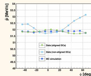
Figure 8: Reconstructed central momentum  $\hat{p}$  vs.  $\phi$  (error bars not visible)
