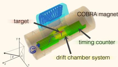
Figure 2:  $e^+$  spectrometer
