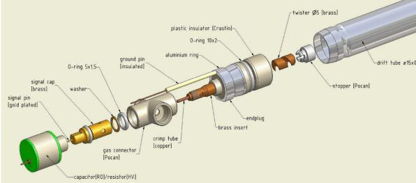
New chamber design similar to the current ATLAS MDT. Main challenge: four times denser tube gas and electrical connections → **new tube endplug** to
