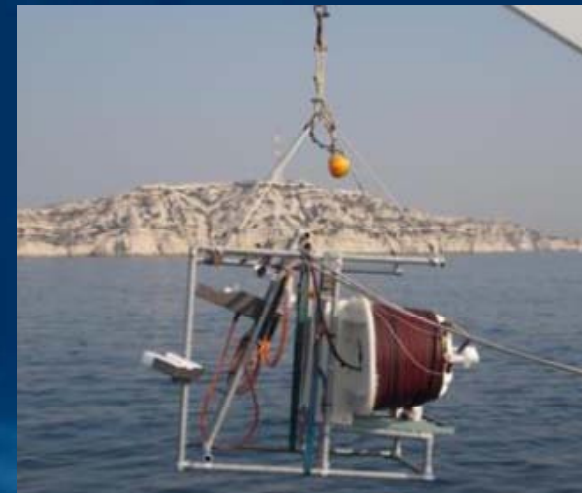
Mock-up of anchor used in test of submarine connection with ROV
