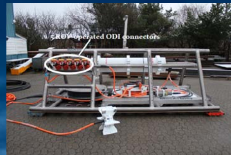
New cable termination frame for KM3NeT-It
