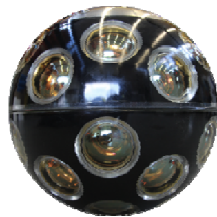
The KM3NeT DOM (31 3" PMTs in a 17" sphere)
