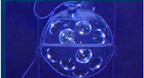
View of one DOM after 1 year in water... (from recent inspection)
