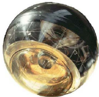
The ANTARES optical module (single 10" PMT in a 17" sphere)
