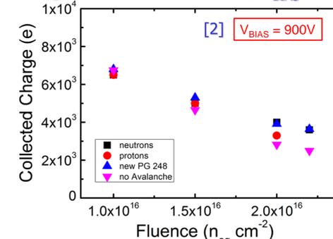
Charge collection at T=248 K,  $V_{BIAS}=900V$
