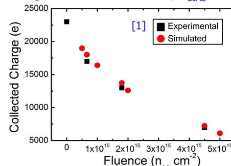
Charge collection at T=248K,  $V_{BIAS}=500V$
