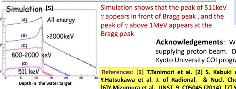
**Result:** Peak position of the higher energy gamma ray image clearly shifts upper position of the beam line. → It is consistent to the simulation result.
