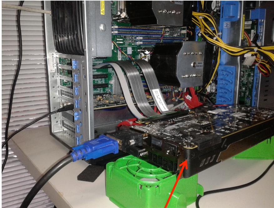
GPU used to test 16-lane PCIe-3 data transfer between the device and the host memory
