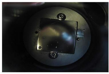
First successful test to deposit multiple layers (0.5  $\mu$ m each) up to ~300  $\mu$ m on a copper backing using the Physical Vapour Deposition (PVD) technique under UHV.
