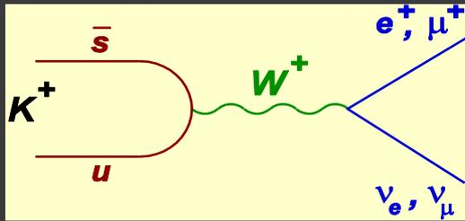
$$R_K = \frac{\Gamma(K^\pm \rightarrow e^\pm \nu)}{\Gamma(K^\pm \rightarrow \mu^\pm \nu)} = \frac{m_e^2}{m_\mu^2} \cdot \left( \frac{m_K^2 - m_e^2}{m_K^2 - m_\mu^2} \right)^2 \cdot (1 + \delta R_K^{\text{rad. corr.}})$$
