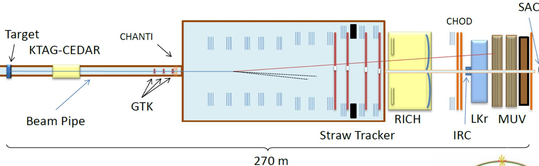
$10^{12}$  / s protons from SPS (400 GeV/c) on Be target ( $\sim 1 \lambda$ )
