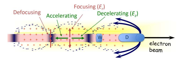
A second, appropriately phased accelerating beam (**witness beam**), containing fewer particles than the **drive beam**, is then accelerated by the wake.
