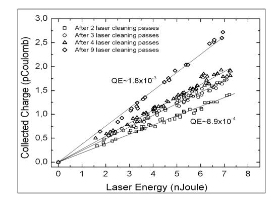
After the laser cleaning, single-photon induces photoemission
