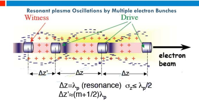
★ Weak blowout regime with resonant amplification of plasma wave by a train of high brightness electron bunches produced by Laser Comb technique
