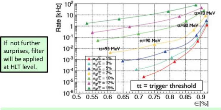
Calorimeter thr = 70 MeV, effi ~ 90 %, DIO rate ~ 2 kHz @ 5 % resol.
