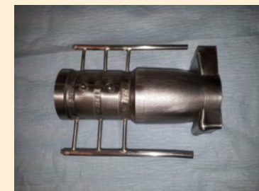
Ni electroformed structure with cooled irises
