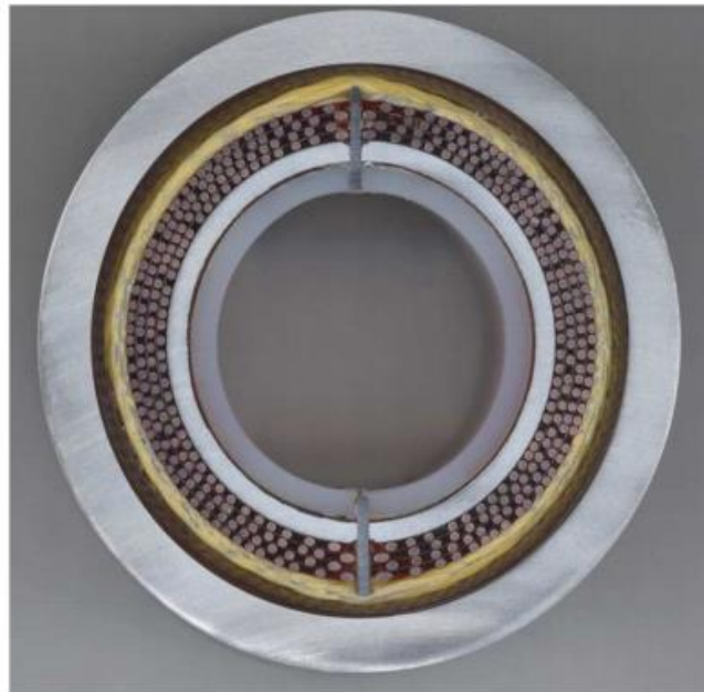
Actual cross section of the dipole tested.
