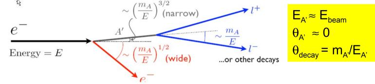
• Vertexing A' decays requires detectors close to the target. Bump hunting needs good momentum/mass resolution. Both need tracking and a magnet.
