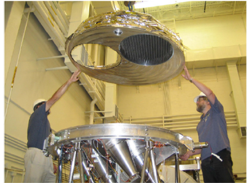
Figure 2. Photograph of the carousel being lowered on top of the aperture plate by two of the authors, showing the porthole for sky viewing and the external calibrator. The carousel turns atop the aperture plate to expose groups of horns to the sky or to the external calibrator. The external calibrator is a blackbody emitter consisting of 298 cones of Steelcast absorber cast onto aluminum cores, and the radiometric side is visible in the photograph. Horn antennas in the core are visible hanging down from the aperture plate.
