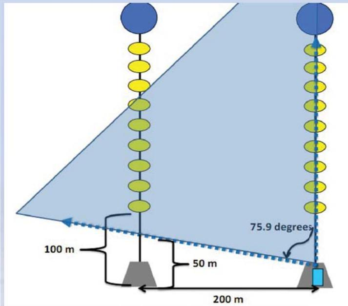
Laser Beacon installed at the base of the NEMO-Phasell tower
