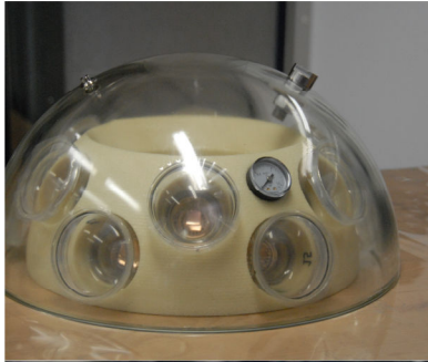
Upper hemisphere with 12 PMTs (mechanical samples), Pressure measurement
