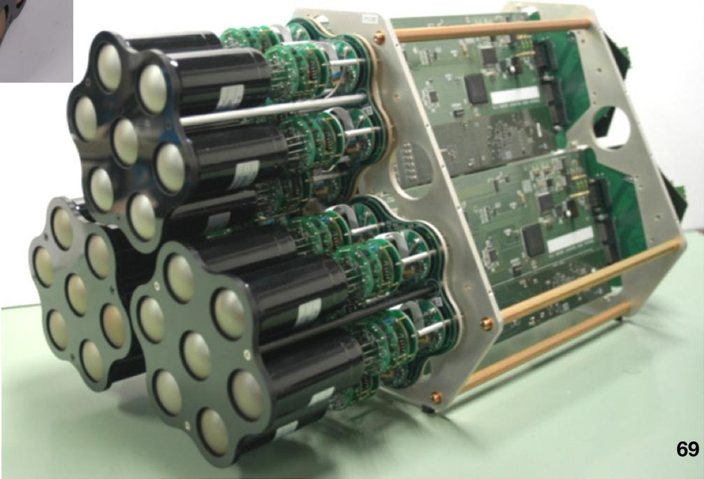
Electronics of the prototype. The contribution from INFN: 50% of the electronics from the PMT to the event formation (Dragon4). Sampling up to 4 GHz
