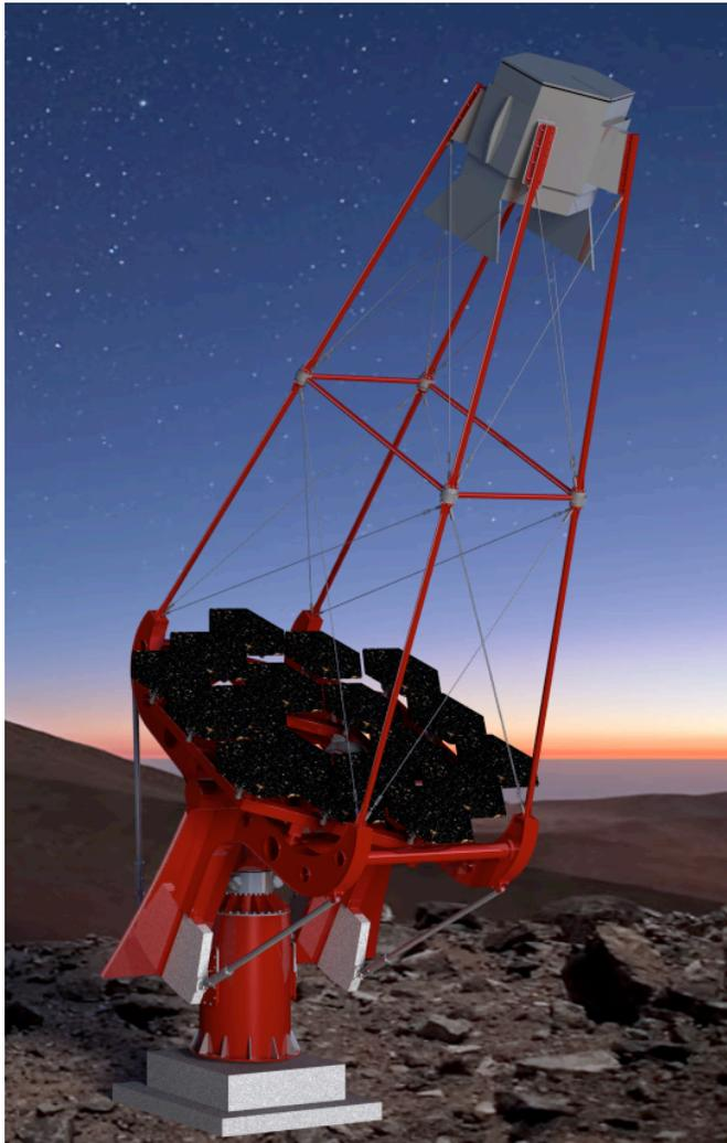
This design is similar to a scaled-down MST and uses the same driving system
