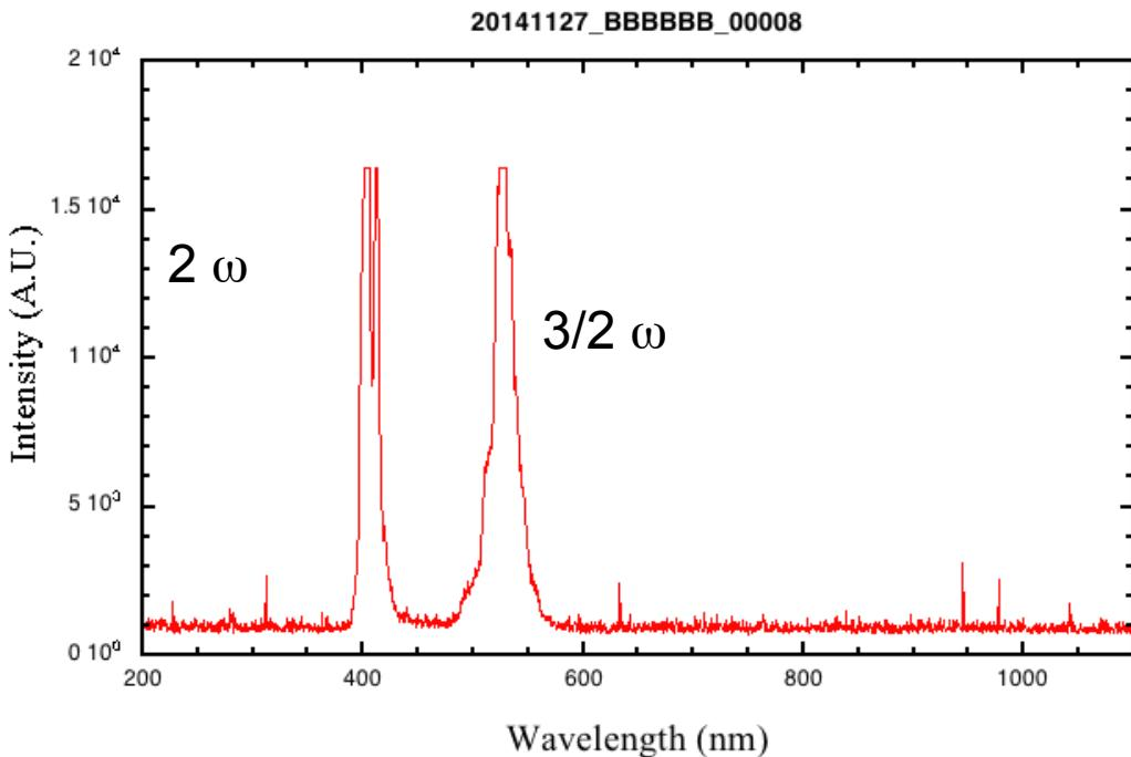
$2\omega_L$  emission => interaction at the critical density layer<sup>&</sup>
