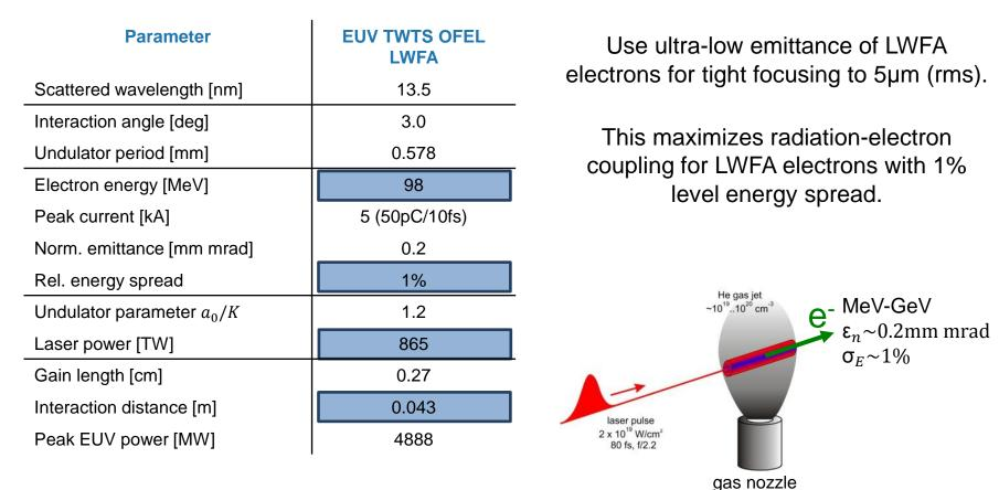
TWTS+LWFA offers inherent synchronization of laser and electrons.
