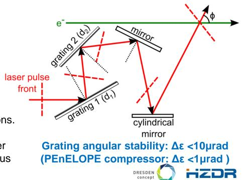
Grating setup can be set up and tested with a low power laser and without electrons.
