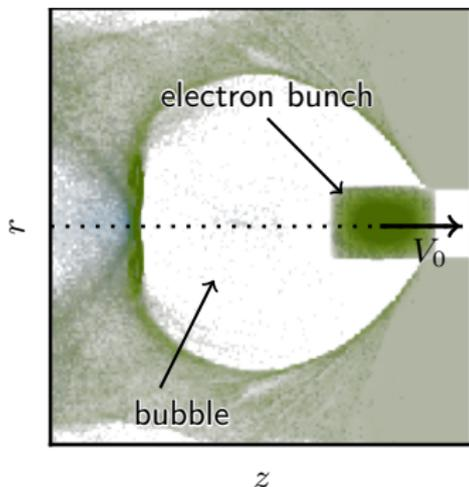
Electron density distribution (green) in a bubble obtained from 3D PIC simulations.
