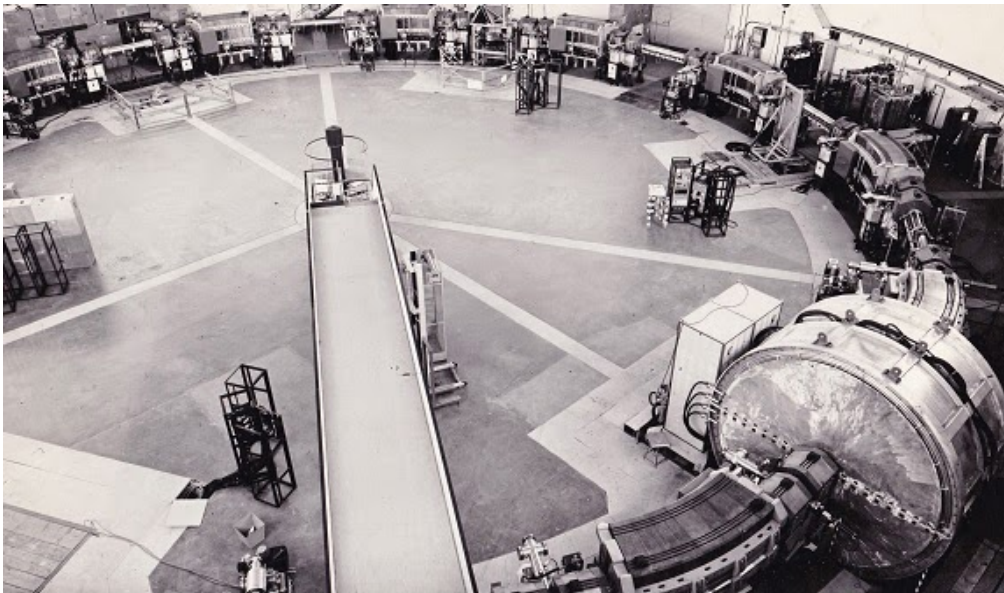
LNF ADONE (big ADA) electron-positron storage ring 1.5 GeV per beam, C = 105 m (1969-1993)
