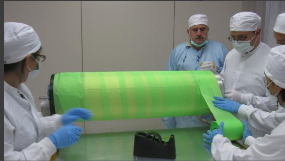
Transpirant tissue (PeelPly from RiBa) is placed around to distribute vacuum
