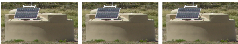
Surface detectors (charged+photon)
