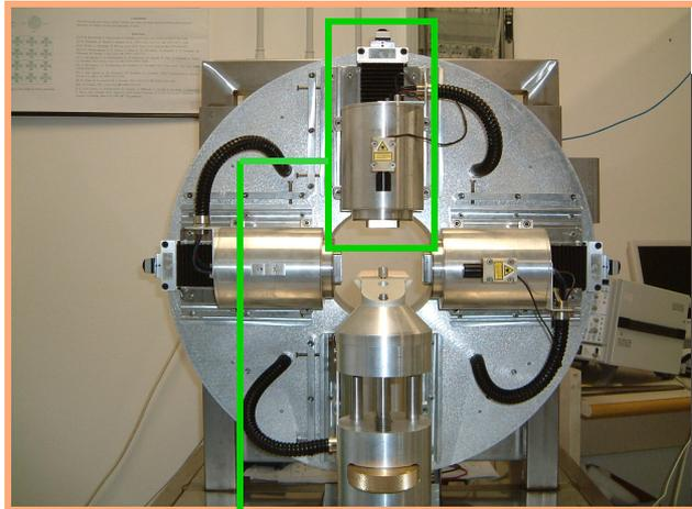
The four heads are mounted on a rotating gantry and the detector spacing can be varied in the 10 cm – 25 cm range (only in our unit).
