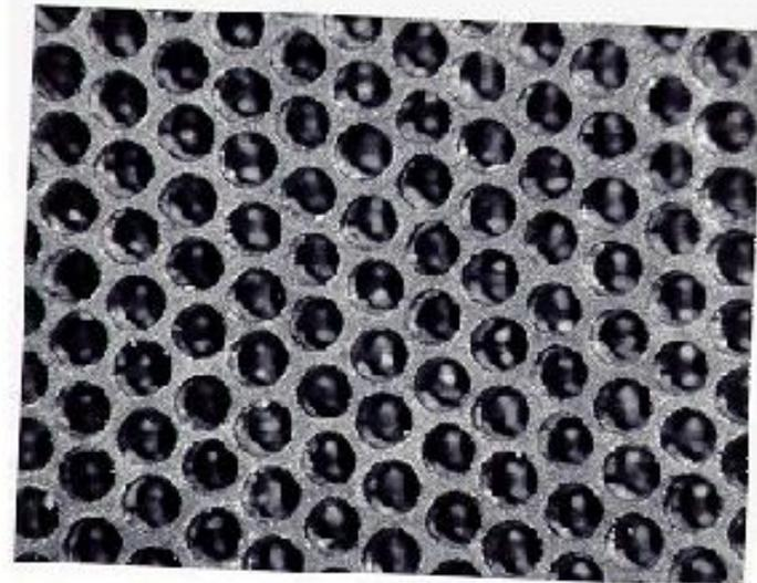
Lead collimator photo: hole diameter 0.6 mm, septa 0.15 mm, height 20 mm.
