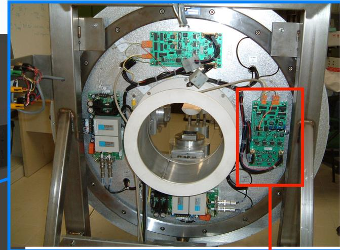
Each acquisition board controls a pair of detectors. It performs the discrimination of the last dynode signals (and the timing coincidence when used in PET mode) using CFD. The four position signals from each tube are sampled and sent to a local PC for the acquisition
