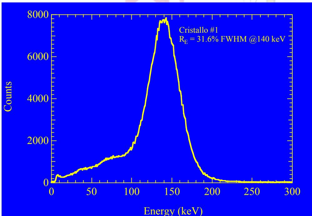
Energy spectra of one of the YAP:Ce matrices (with collimator) after having applied energy corrections to each single crystal pixel.
