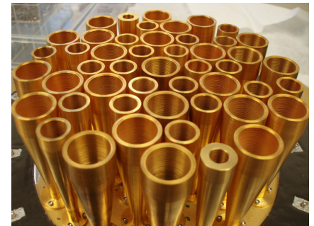
BICEP1: Feedhorns and NTD readout 150 and 100 GHz
