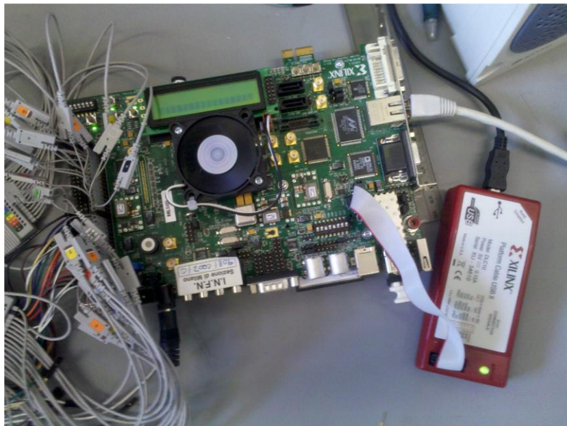
Figure 4: FPGA evaluation board to perform LAr trigger studies
