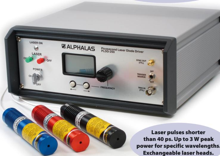
Laser pulses shorter than 40 ps. Up to 3 W peak power for specific wavelengths. Exchangeable laser heads.
