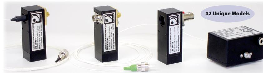
The UPD series of ultrafast photodetectors are best suited for measurement of optical waveforms from DC to 25 GHz. Various models feature rise times as short as **15 ps** and cover the spectral range from **170 to 2600 nm**.
