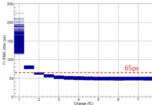
$T_1(\text{RMS}) < 65 \text{ ps at } 2.5 \text{ fC}$
