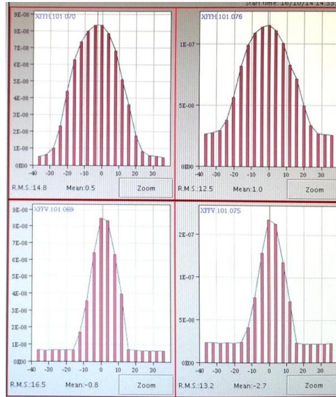
Horizontal (top) and vertical (bottom) profiles before (left) and after (right) the KTAG counters measured with FISC counters. These profiles are now symmetric as expected
