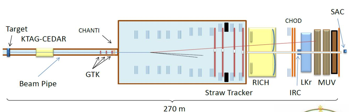
$10^{12}$  / s protons from SPS (400 GeV/c) on Be target ( $\sim 1 \lambda$ )
