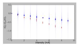
No TMCI observed around 8.8 mA. Indication for missing impedance contribution/s
