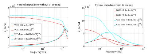
Much better agreement between CST and IW2D without the Ti coating. Factor of 2 difference in the case of Ti coating
