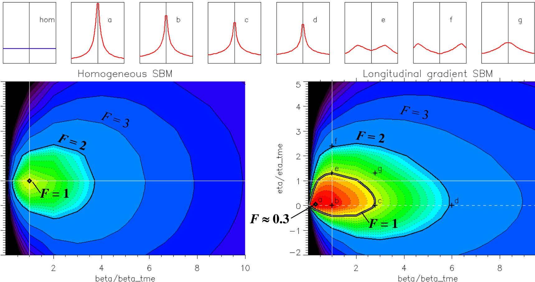
small (~0) dispersion at centre required, but tolerant to large beta function
