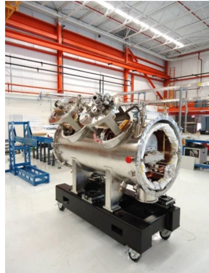
Fit test of cold mass and current lead assemblies in cryostat
