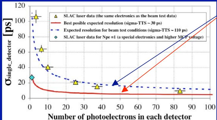
$$\begin{aligned} \sigma &\sim \sqrt{[\sigma_{\text{MCP-PMT}}^2 + \sigma_{\text{Laser}}^2 + \sigma_{\text{Electronics}}^2 + \dots]} = \\ &= \sqrt{[\sigma_{\text{TTS}}/\sqrt{N_{\text{pe}}})^2 + \sqrt{((\text{FWHM}/2.35)/\sqrt{N_{\text{pe}}})^2 + (4.2 \text{ ps})^2}] } \end{aligned}$$
