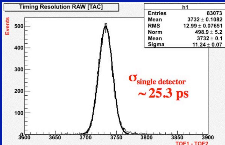
Fermilab beam test, 120 GeV p:
