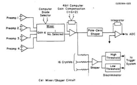
Schematic of the mixer/shaper circuits between the crystal preamplifiers and the ADC's.
