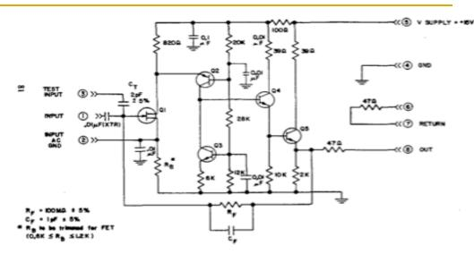
38 Circuit diagram of the preamplifier connected to the silicon photodiode.
